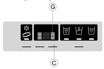
To switch off the refrigerator, press and hold button C for a few seconds. The icon (G) will disappear.
